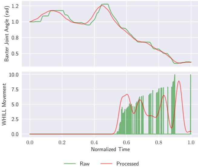
Fig. 4: Preprocessing of the collected data. We use the median filter and cubic interpolation to preprocess the collected data. We are showing only one joint angle of the Baxter robot. The WHILL movement refers to the forward tilt of the joystick.
