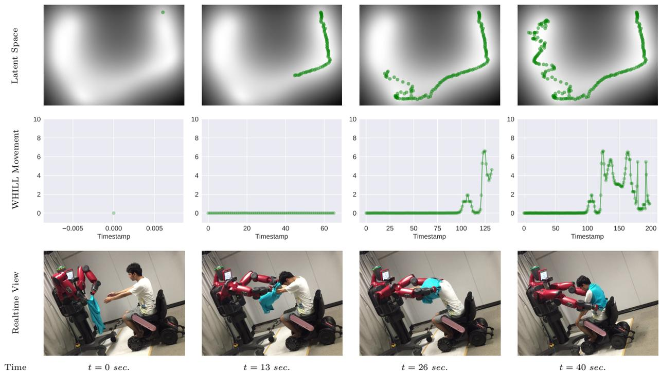
Fig. 8: The clothing assistance task with Baxter and WHILL shown at various timestamps. The mean trajectory in latent space is sampled and shown in Green color in the latent space.
