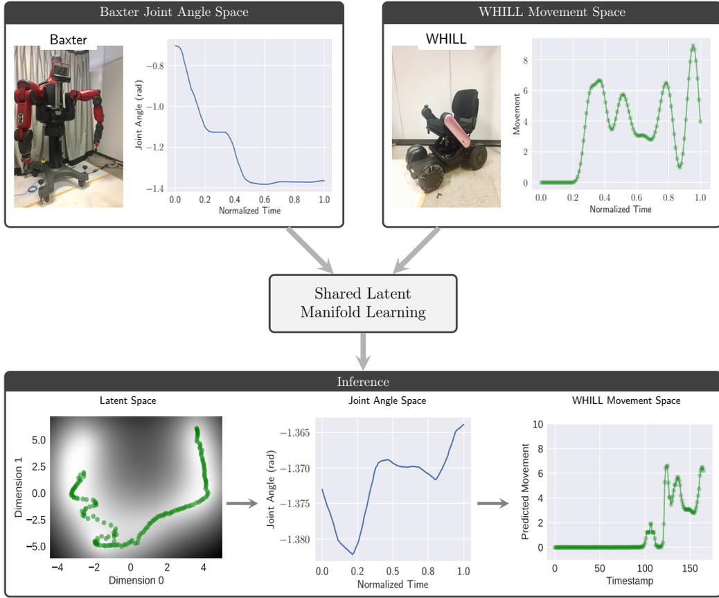
Fig. 2: An overview of the proposed method for the collaboration between Baxter and WHILL. We defined two observation spaces, i.e., Baxter joint angle space (only 1 of the 14 joint angles of the robot is indicated in the graphs here) and WHILL movement space, and learned a shared latent space by employing MRD.
